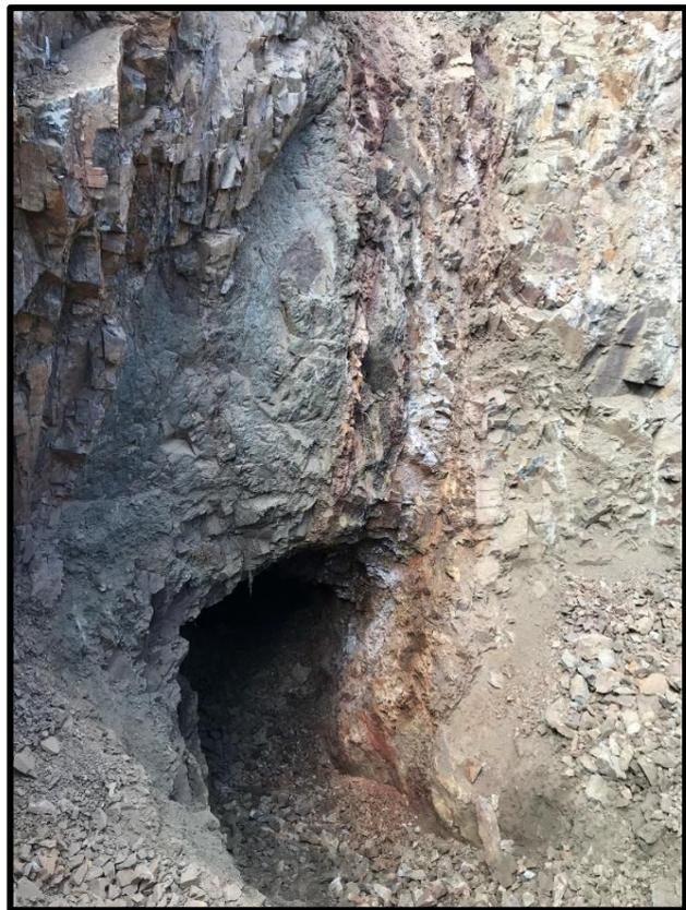
**Figure 4: Gold bearing quartz vein on right**
